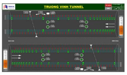
Emergency response also relies on the SCADA system, using visibility sensors to detect accidents or incidents in real-time, facilitating swift responses by emergency teams, thus contributing to improved safety for all tunnel users.
