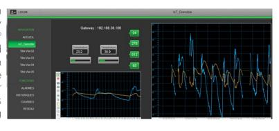
The integration of the LoRaWan network at the heart of the GTB PcVue solution allows feedback from sensors used with the existing BMS supervision. The "raw" data of the sensor (Temperature, On / Off) is enhanced by the power of PcVue to enrich and treat this data including, creation of threshold, alarms, mimic, curves and archiving.
