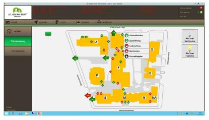
This also relieves the staff, doors no longer must be locked manually, unexpected visitors have no access and the technician on site has an easier time managing the building. During the next round of door maintenance, a check is made to see which door systems can be connected to the PcVue system with little effort using BACnet. This simplifies to connect the subsystem "doors" step by step.
